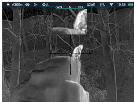
with a short press of the **Zoom (4)** button, the PIP image will be enlarged 2× synchronously.
